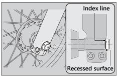
4. Tighten the left axle pinch bolts.
