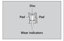
Inspect the brake pads from the bottom of the brake caliper.
