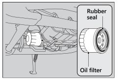
**7.** Apply a thin coat of engine oil to the rubber seal of a new oil filter.
