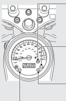
(B) ABS (Anti-lock Brake System) indicator VT750CS Comes on when the ignition switch is turned to the ON position. Goes off when your speed reaches approximately 6 mph (10 km/h)
