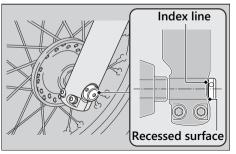
4. Tighten the left axle pinch bolts.
