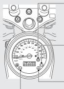
ABS (Anti-lock Brake System) indicator VT750CS Comes on when the ignition switch is turned to the ON position. Goes off when your speed reaches approximately 6 mph (10 km/h)
