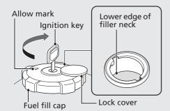
Do not fill with fuel above the lower edge of the filler neck.
