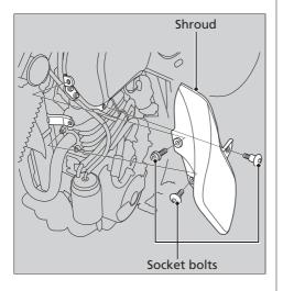
The shroud must be removed for access to the spark plug.
