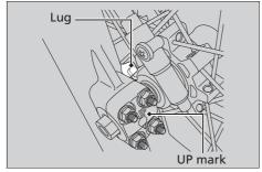
**4.** Tighten the front axle shaft.
