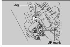
**4.** Tighten the front axle shaft.
