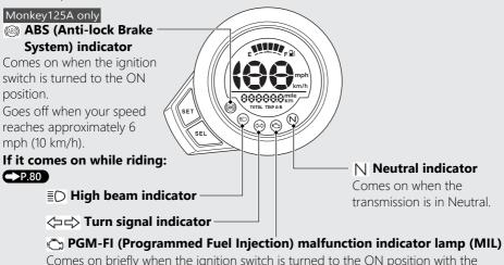
Comes on briefly when the ignition switch is turned to the ON position with the engine stop switch in the  $\bigcirc$  (Run) position.
