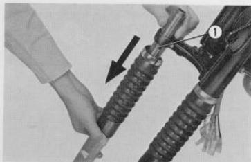
Fig. 4.20 Removing front cushion
