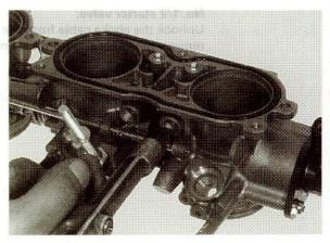
Remove the starter valve shaft, three collars and return spring.
