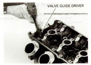
Ream the new valve guide after installation. Insert the reamer from the combustion chamber side of the head and also always rotate the reamer clockwise.
