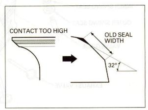
If the contact area is too low on the valve, the seat must be raised using a 60-degree inner cutter.
