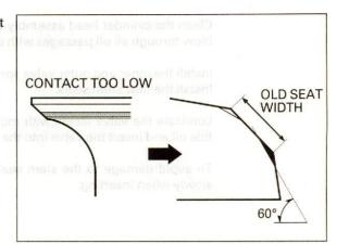
Refinish the seat to specifications, using a 45degree finish cutter.
