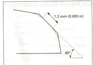
Apply a thin coating of Prussian Blue to the valve seat.
