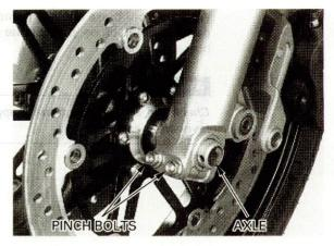
Hold the axle and tighten the axle bolt to the specified torque.
