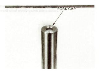
Hold the damper rod lock nut with a 14 mm spanner, then loosen and remove the fork cap from the damper rod.
