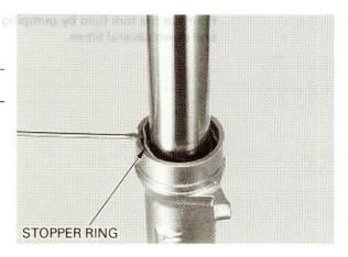
Pull the fork tube out until you feel resistance from the slider bushing. Then move it in and out, tapping the bushing lightly until the fork tube separates from the fork slider.
