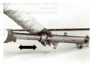
Remove the oil seal, back-up ring and slider bushing from the fork tube.
