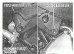
Remove the rear/upper engine hanger bolt, distance collars and spacer.
