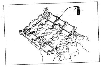
Install the camshafts onto the cylinder head with their cam lobes at the No.1 cylinder facing up as shown.
