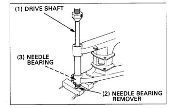
Press a new needle bearing with the stamped side facing out.
