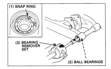
Press new radial ball bearings into the right swingarm pivot one at a time.
