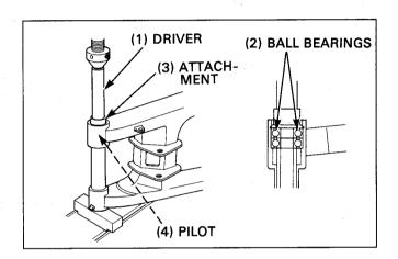
Press the needle bearing out of the left swingarm pivot.
