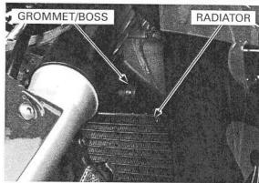
Install the horn mounting stay, washer and radiator upper mounting bolt.
