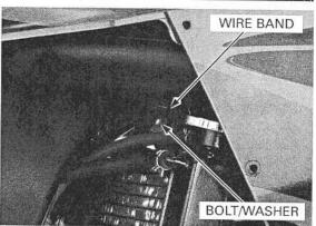
Install the radiator lower mounting bolt, washer and nut.
