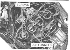
Install the upper air cleaner housing and eight screws.
