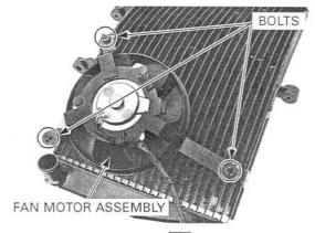
Remove the nut and cooling fan.
