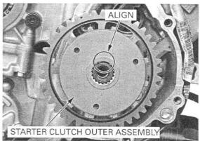
Apply oil to the starter clutch outer special bolt threads and seating surface.
