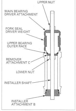
Install the special tools into the steering head pipe as shown.
