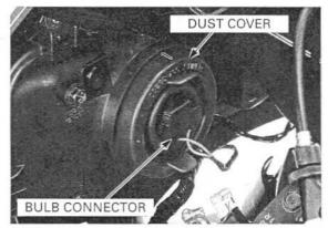
Unhook the bulb retainer and remove the headlight bulb/socket.
