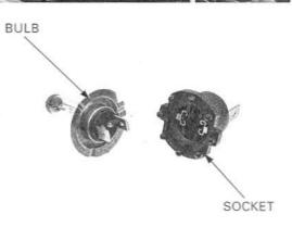
Install the new headlight bulb/socket aligning its tab with the groove in the headlight unit.
