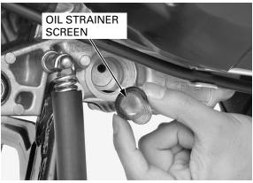
Make sure the O-ring is in good condition and replace it if necessary.
