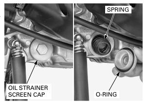
Remove the engine oil strainer screen.
