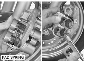
Always replace the brake pads in pairs to assure even disc pressure.
