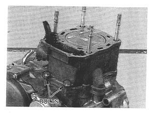
Remove the gasket and dowel pins.
