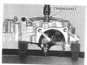
Remove the left crankshaft bearing using a bearing puller.
