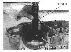
Install the new right crankshaft oil seal.
