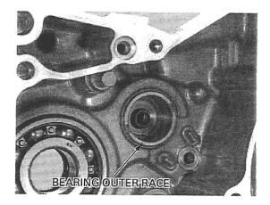
Clean the outer race stopper plate bolt threads and apply a locking agent to bolt threads. Install and tighten the stopper plate bolt securely.
