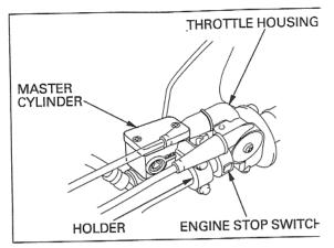
Remove the screw and throttle cable roller cover. Remove the cable roller.
