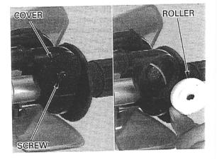
Remove the screws and throttle housing cover.
