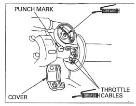
Apply grease to the sliding area of the cable roller and insert it into the throttle housing.
