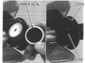
Install the left handlebar switch housing onto the handlebar, aligning the locating pin with the hole in the handlebar.
